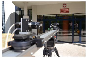
The system itself is very simple. It consists of a pair of cameras, rigidly connected to each other, forming a stereoscopic system. The data processing is done on a personal computer using dedicated software. This simple stereoscopic system, situated next to a road, allows to reliably detect all oversized vehicles.
