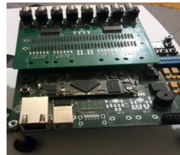
Figure 7. Board with FPGA and D/C converters
