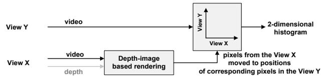
Fig. 4. Scheme of the experiment for disparity-based pixel correspondence noise analysis..
