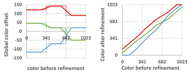
**FIGURE 4.** Left: exaggerated example of global color offsets for 3 color components, with (solid line) and without (dotted line) range overlapping. Right: color transform functions for 3 color components.
