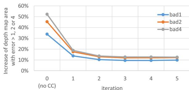
FIGURE 14. Decrease of the number of pixels with depth error higher than 1, 2, or 4 disparity levels over consecutive iterations; the number of pixels shown as an increase of area with wrong disparity compared to depth maps estimated using color-consistent views.
