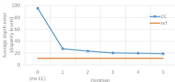
FIGURE 13. Average depth error in depth maps estimated using color-consistent views (orange line) and non-consistent views without and with color refinement (blue line).
