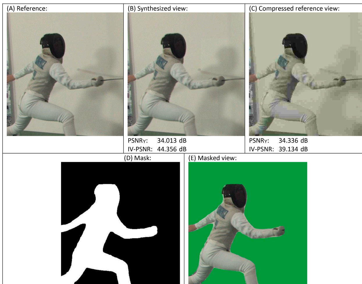
Fig. 4. Fragments of a single view (v8), Fencing sequence. A: reference view, B: view v8 synthesized using views v7 and v9, C: reference view heavily compressed with JPEG, D: binary mask (used in masked mode), E: masked view (green area excluded from quality assessment in masked mode).
