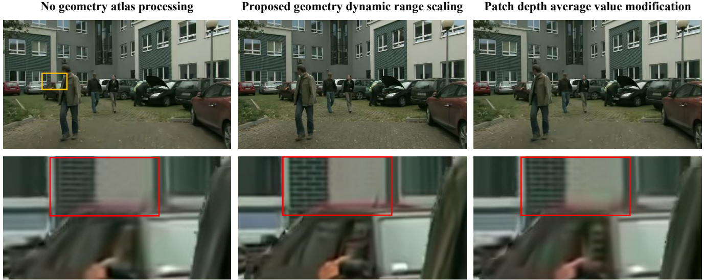
Fig. 11. A viewport (and its fragment) synthesized using atlases processed in 3 ways; left: no geometry atlas processing, center: proposed (geometry dynamic range scaling), right: patch depth average value modification; natural content – sequence Carpark [52].
