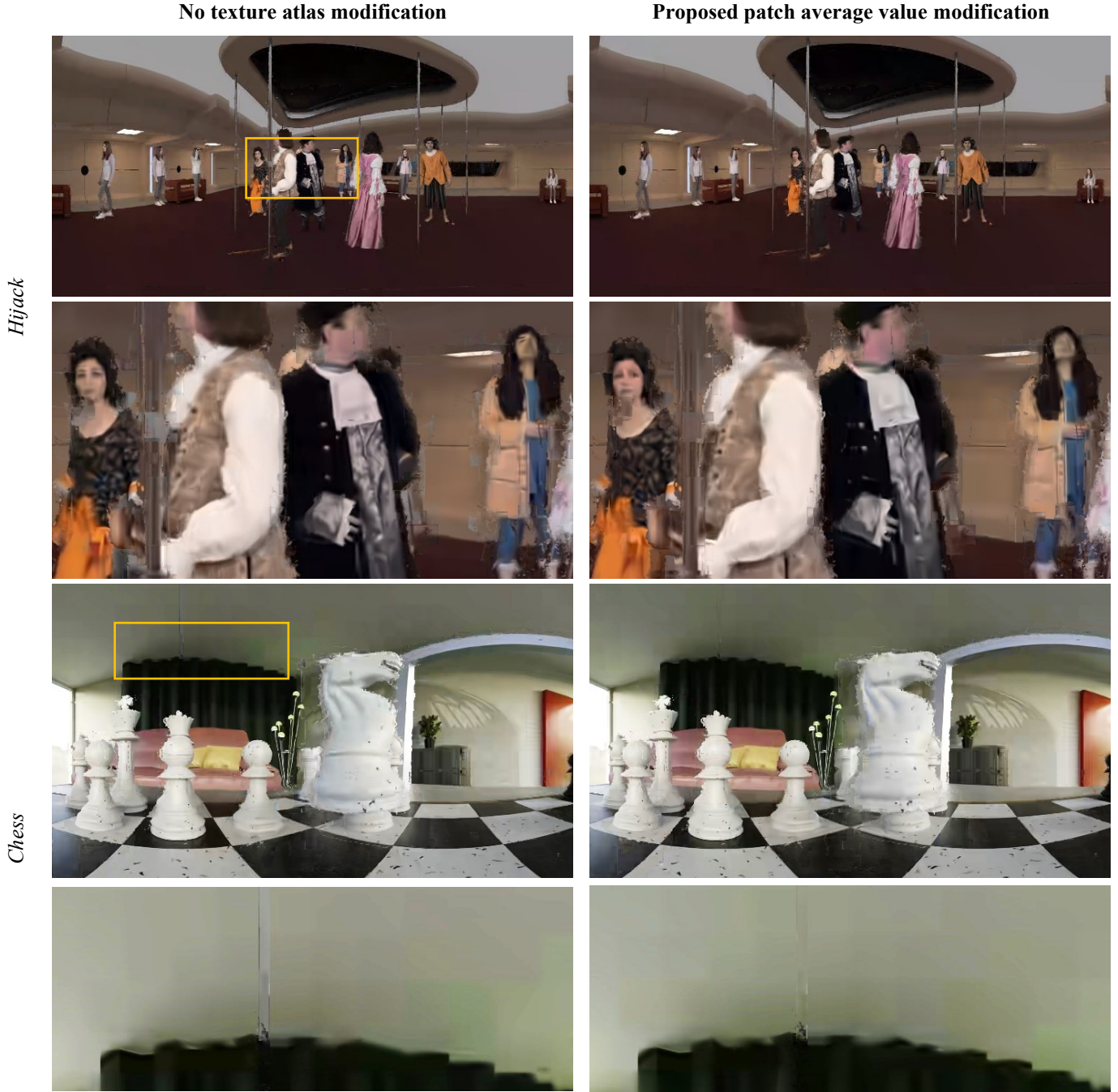
Fig. 16. A viewport (and its fragment) synthesized at a very low bitrate; many occlusions ( Hijack [41]) and smooth area ( Chess [37]).
