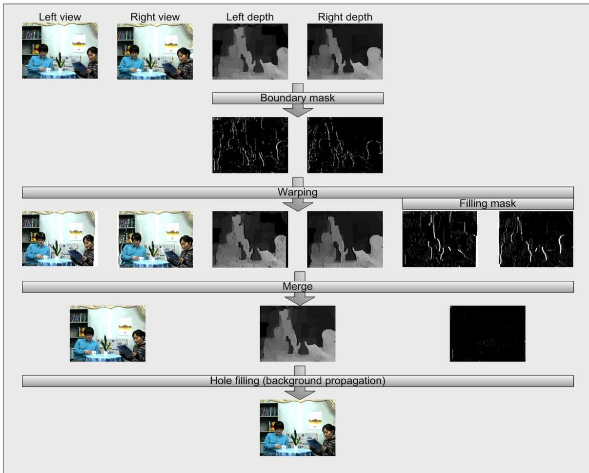
**Figure 36: Flow diagram for VSRS 1D mode.**
