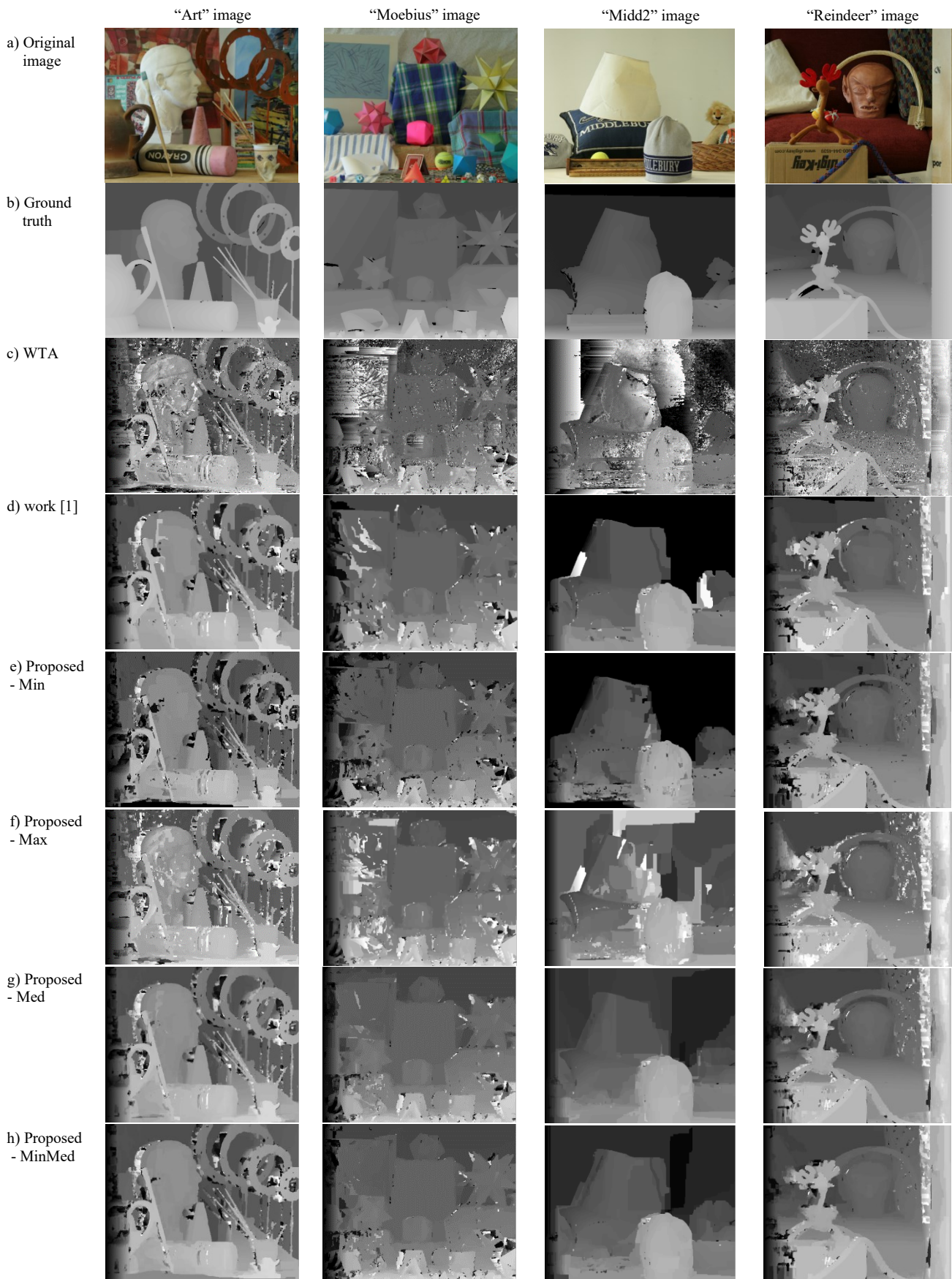
Fig. 5. Experimental results – “Art” and “Moebius” images from Middlebury dataset [15]: a) the original image, b) ground-truth depth map, c) Winner Takes All (WTA) technique, d) technique from work [1], e) proposed – Min, f) proposed – Max, g) proposed – Med, h) proposed – MinMed.
