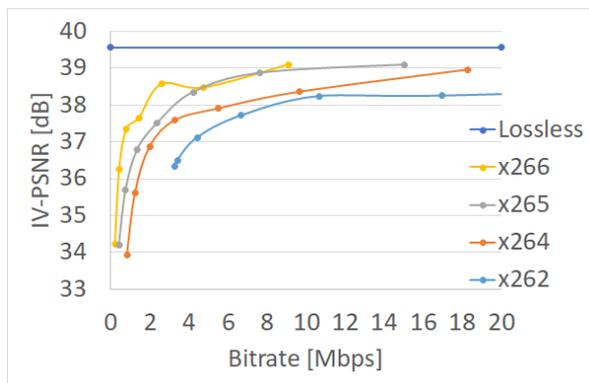
Figure 11: IV-PSNR rate-distortion curves for synthesized virtual views.
