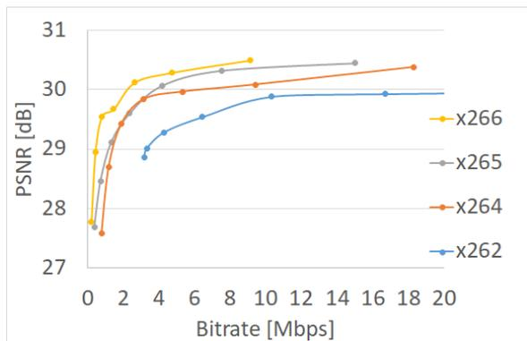
Figure 10: PSNR rate-distortion curves for decoded source views.
