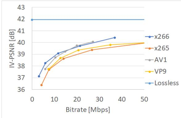
Figure 4: IV-PSNR rate-distortion curves for synthesized virtual views.
