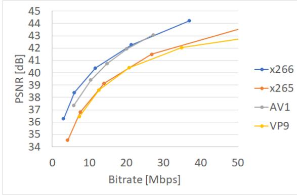
Figure 3: PSNR rate-distortion curves for decoded atlases.
